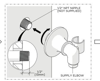
2. Ensure the 1/2" NPT NIPPLE (not supplied) projects 1/2" [13mm] from the surface of the finished wall then thread and securely tighten the SUPPLY ELBOW onto the NIPPLE.
