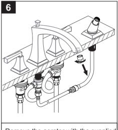
Remove the aerator with the supplied key. Turn the water supply on.
