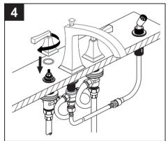
Place the "O" ring over the cold valve. Align the handle and place the handle and escutcheon assembly into the valve. Secure the assembly by turning the escutcheon clockwise. Repeat for hot valve.
